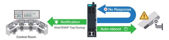
Moxa's Smart PoE switches can detect unresponsive PDs and automatically trigger recovery actions based on user-defined parameters—helping reduce downtime and avoid unnecessary site visits.
